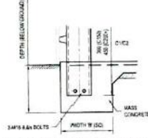
ALTERNATIVE COLUMN IN GROUND DETAIL #3 1:20
